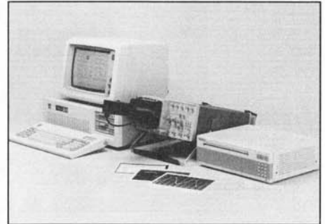
DCS01 Digitizing Camera System captures repetitive waveforms from analog scopes and transients according to a scope's CRT writing speed (350 MHz for 2467).
