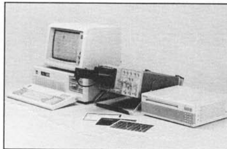
DCS01/2467 Digitizing Camera System captures repetitive waveforms and transients from analog scopes according to a scope's CRT visual writing speed (2467: 4 div/ns).
