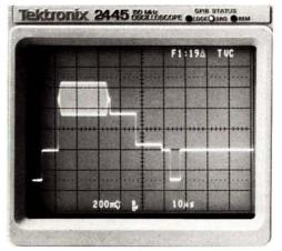
This sample waveform and CRT readout show a 2445's highfidelity display of the Vertical Interval Reference Signal on Line 19, Field 1 with the television blanking-level clamp (TVC) engaged. The instrument used is also equipped with Option 10 (GPIB).
