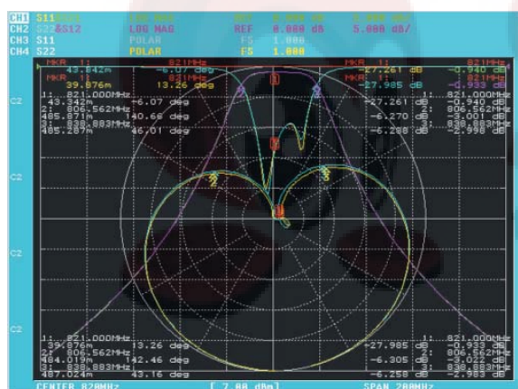
4-channel, 6-trace display with ANNOTATION ON, MENU OVERLAY OFF, SCALE UP OFF
