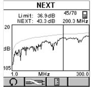
Above: OMNIScanner displays a NEXT graph for each pair combination. Limit and NEXT are shown for the frequency indicated by the cursor position.
