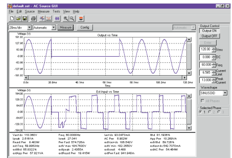
Testing of UPS Input and Output using Dual Power Analyzer Option 020
