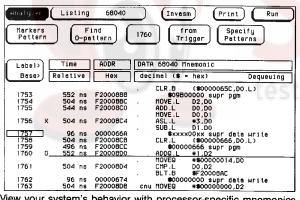
View your system's behavior with processor-specific mnemonics, using HP preprocessors and inverse assemblers.
