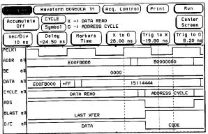
Make timing measurements with up to 2-ns resolution. Display bus values inside the waveforms, using any base (including symbols).
