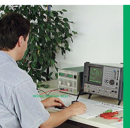
Built-in spectrum analyzer AUTORUN IEEE-488 interface High-speed measurements Reliability In excess of 5000 STABILOCK 4032 radio test sets are currently in use worldwide. This success has been due to the versatile design, simple operation and wide variety of system tests which can be made with the "universal" test set.
