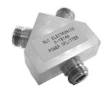
RLC Electronics' D—1814A is a broadband DC to 18 GHz resistive power splitter which utilize two resistors, one on each of the output ports, and is a unidirectional device. It provides exceptional amplitude tracking and a very low
