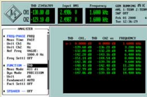
Fig. 11: Complete measured-value tables can be output for all functions.
