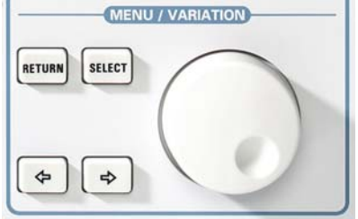
FIG 10: General settings and menu selection with spinwheel, RETURN, SELECT and arrow keys
