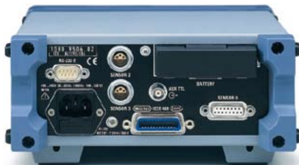
The battery, the R&S® NAP sensor connector and two R&S® NRT sensor connectors are accessible on the rear panel
