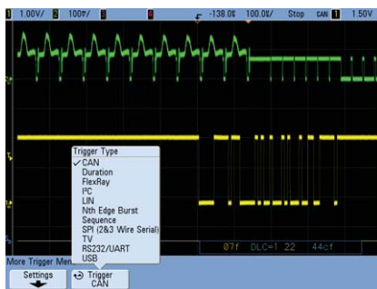
Trigger on and decode CAN serial packets.
