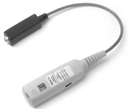
Figure 5. The Agilent E2621A ac-coupled, balanced adapter allows connection to differential communications signals by terminating the signal into 100, 110, or 120 ohms.
