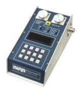
The Model 4319A is a Rugged RF Power Analyst that monitors Peak Pulse Power, Peak Envelope Power, or CW Power during normal equipment operations in the forward or reflected direction. Designed for air navigational aids DME, ATC and other pulsed RF systems such as telemetry, radar, commandand control, etc. They need no attenuators, directional couplers or charts.
