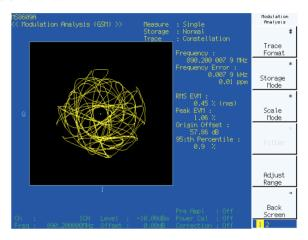
The following screen shows the constellation display for the 8PSK modulation through a Nyquist filter and Gaussian inverse correction filter.
