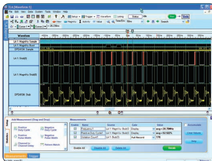
► Tektronix' Integrated View feature (iView™) fully integrates the performance and measurement accuracy of a Tektronix oscilloscope with the multi-channel and powerful triggering capabilities of a Tektronix logic analyzer in one display, allowing designers to quickly verify and debug their designs.
