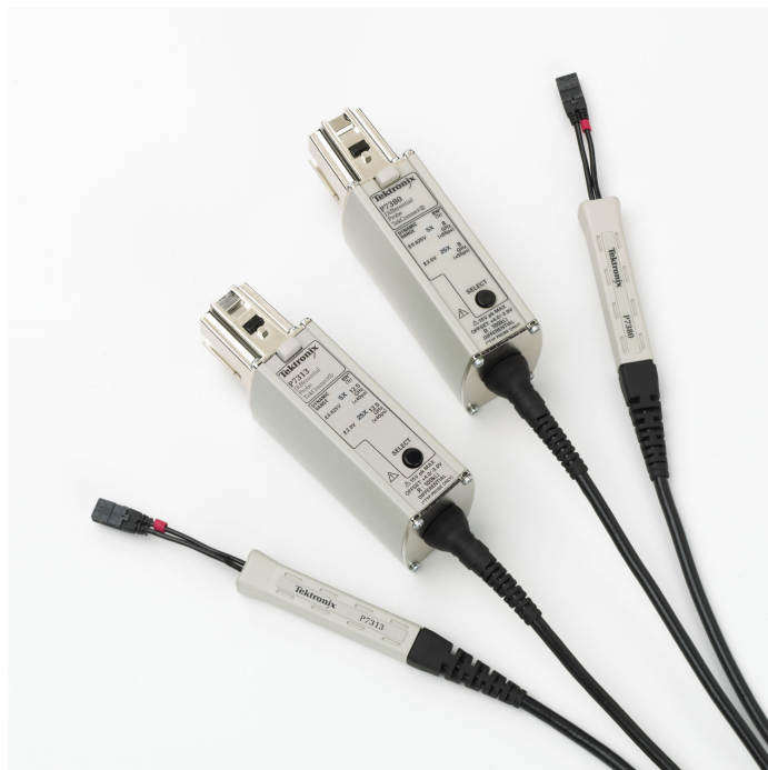
P7313 12.5 GHz and P7380 8 GHz Differential Probes.
