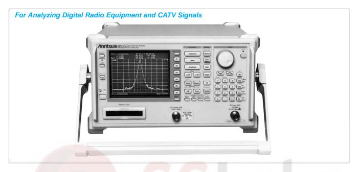
The MS2661C Portable Spectrum Analyzer is for signal analysis of radio and other equipment related to improving frequency usage efficiency, higher modulation, and digitalization. This is a synthesized spectrum analyzer covering a wide frequency range from 9 kHz to 3 GHz. It has superior basic performance such as high C/N ratio, low distortion, and high frequency/level accuracies and is easy to operate.
