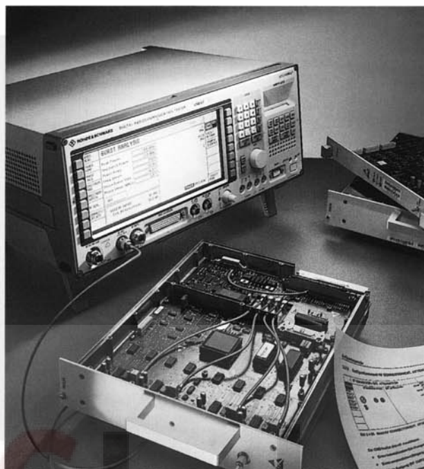
Typical test setup in module production: CMD 54/57 is remote-controlled via the IEC/IEEE bus, while the DUT is controlled via a manufacturer-specific bus
