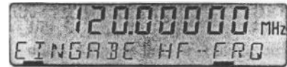
Alphanumeric display as communication aid between test set and user. Here: request to enter RF frequency of receiver
