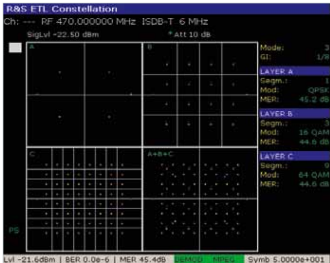
Constellation diagram of an ISDB T signal with excellent MER.
