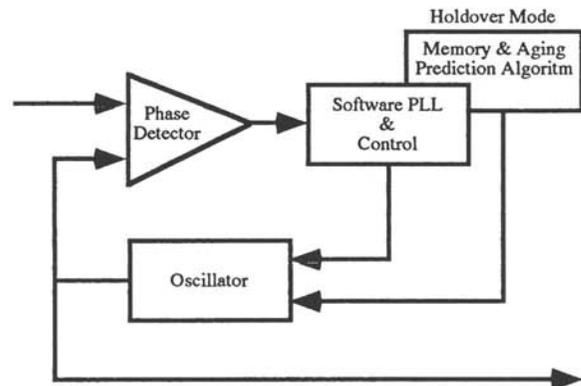
Figure 1. HP SmartClock Concept
