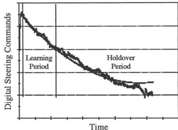
Figure 2. Typical HP SmartClock Holdover Aging Performance
