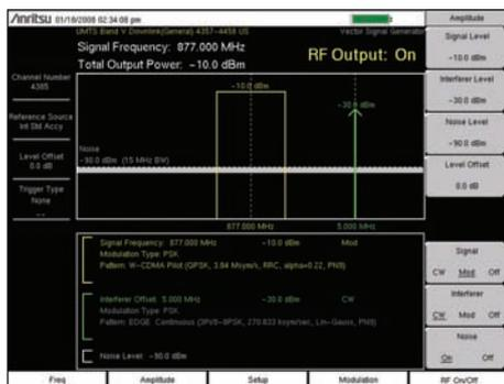
**Intermodulation Rejection Test Set-up**
