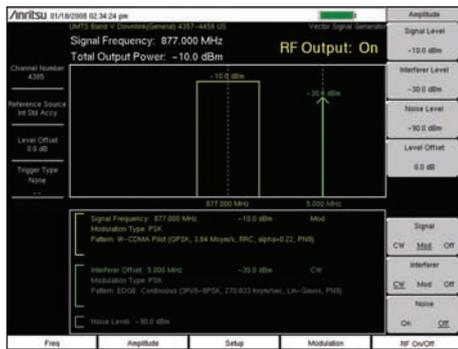
**Sensitivity Test Set-up**
