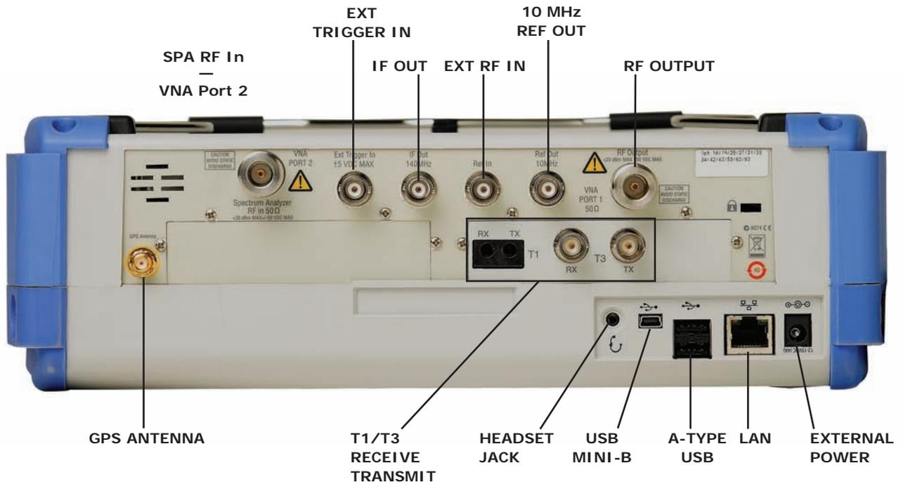
All Connectors are conveniently located on the top panel, leaving the sides clear for handheld use
