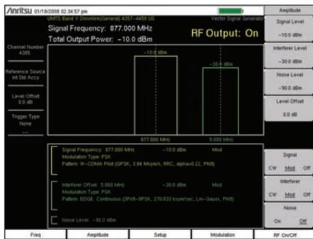
**Blocking Test Set-up**
