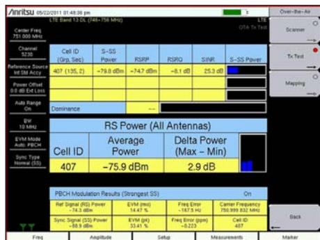
**Over-the-Air Measurements – Tx Test**
