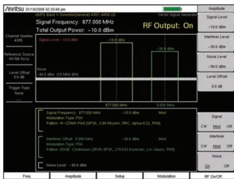
**Adjacent Channel Selectivity Test Set-up**
