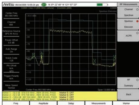
**RF Measurements – Spectral Emissions Mask**
