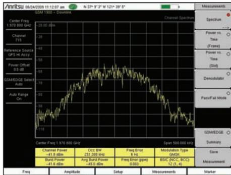
**RF Measurement – Occupied Bandwidth**
