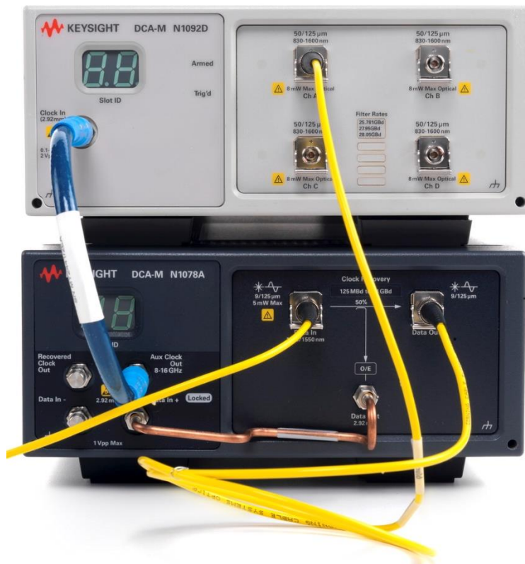
N1078A Clock Recovery triggering a N1092D DCA-M
